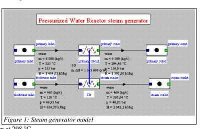
The feedwater from the secondary circuit enters the GV at 47 bar and *Figure 1: S* 150 °C, and leaves as superheated steam at 298 °C.
