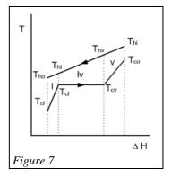
If the fluid enters the evaporator in the two-phase state, the equations are slightly different.
