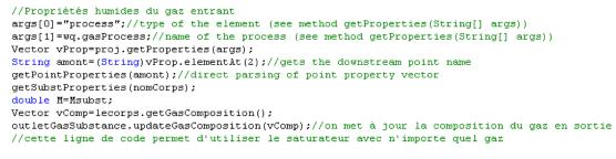
2) we calculate the inlet absolute humidity with the definition formula, to avoid, given the high temperature of gas, having to estimate the saturation conditions.
