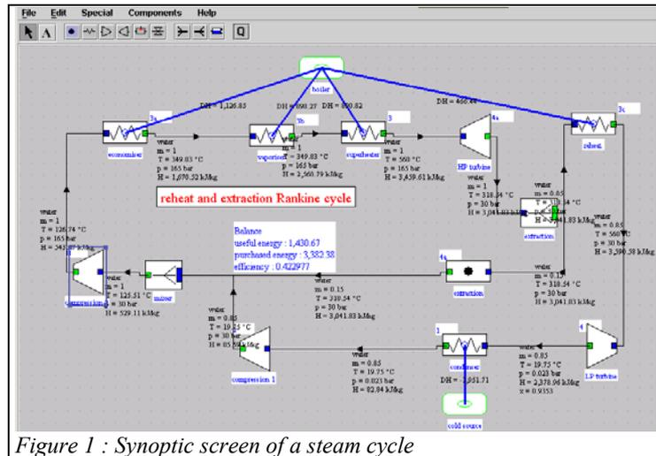
Figure 1 : Synoptic screen of a steam cycle
