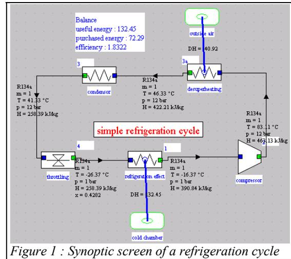
Figure 1 : Synoptic screen of a refrigeration cycle
