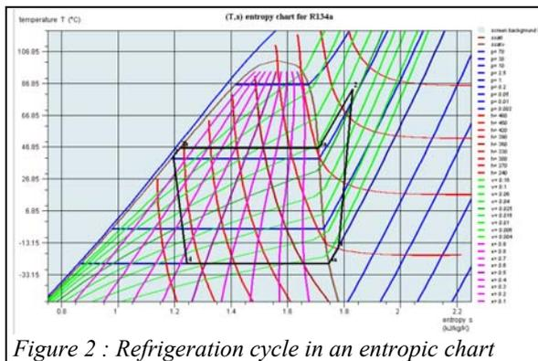
Figure 2 : Refrigeration cycle in an entropic chart
