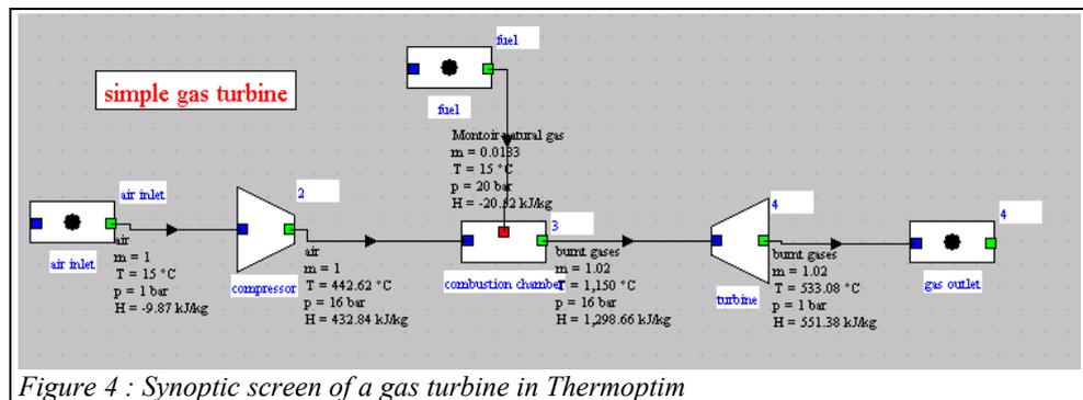
Figure 4 : Synoptic screen of a gas turbine in Thermoptim
