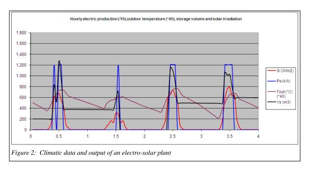
This model is very simplified since it does not take into account the heating of the collector field in the morning (more precisely, it does not take it into account explicitly, but the collector heats up as the sun remains below the positive efficiency threshold).
