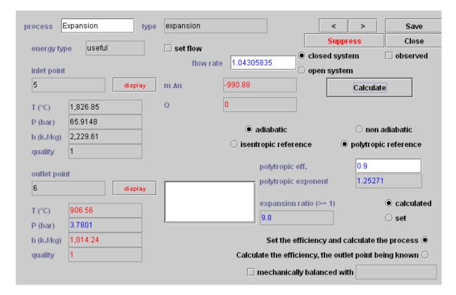
This is "closed system" expansion with a calculated expansion ratio. The isentropic efficiency here is set equal to 0.9. The pressure at the expansion outlet is equal to 3.78 bar, the temperature to 906.5  $^{\circ}$ C, and the expansion work is equal to 991 kJ.
