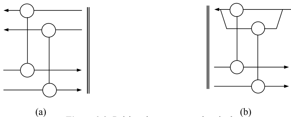
Figure 3.8: Pairing the streams at the pinch
