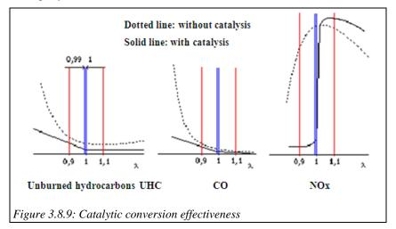
It is for this reason that the use of a "three ways" catalytic converter can only be justified with a very precise control of fuel and combustion, that is to say with injection and electronic ignition control devices of the type we presented above.
