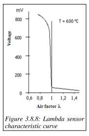
With the catalysts, it is possible to combine these different operations, but with the imperative of fully controlling the oxygen dosage, which can be done thanks to the Lambda sensor because of its very steep voltage characteristic for  $\lambda = 1$ .
