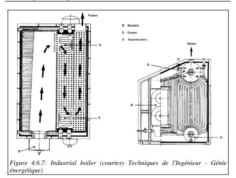
However, the former are limited to capacities lower than the latter, for reasons of mechanical strength and safety (with a very large volume of water under pressure). Their main area of use is the supply of saturated steam under low pressure (<15 bar), and represent over 60% of the French fleet of boilers, against 20-25% for water tube boilers, which are well suited for the supply of superheated steam at medium and high pressure.
