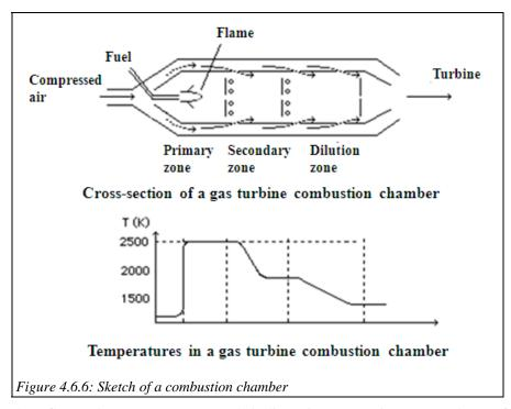
These flame tubes are very compact, their dimensions amounting to several tens of centimeters at most. Subjected to intense and high temperature heat fluxes, the materials they contain are resistant steel sheet potentially coated with ceramic.
