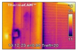
Thermal photo is a useful way to detect thermal bridges.
