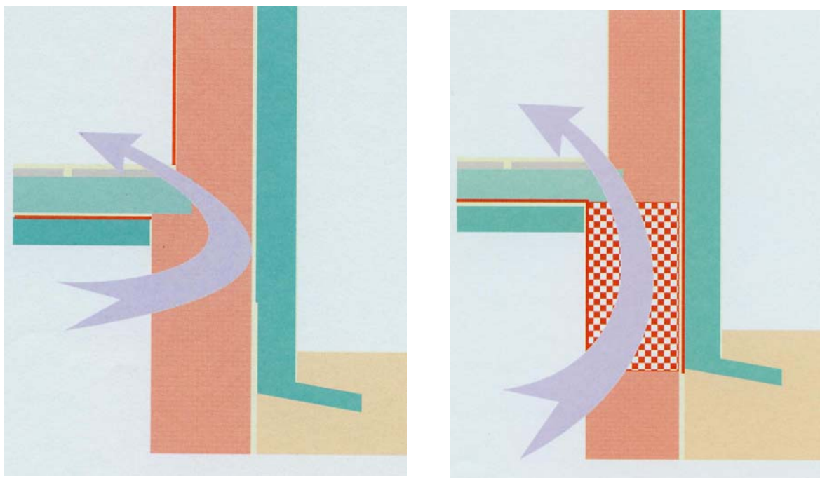
Fig. 4: Remaining weak point at the cellar brickwork
