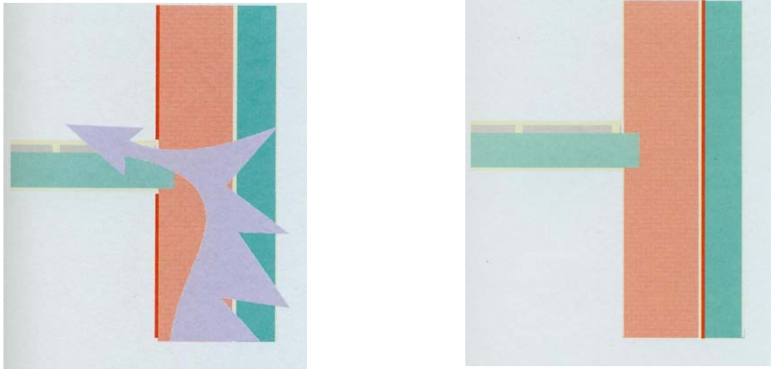
Fig. 3: transferring of the airtightning layer from inside to outside plaster of external wall
