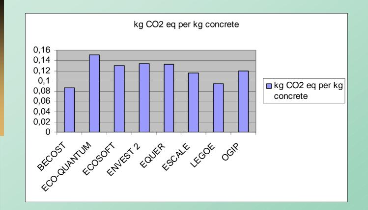
Different qualities, cement content 120-300 kg/m<sup>3</sup> Different processes (prefabricated) and energies Different indicators : IPCC, CML... + alloc. (ash)
