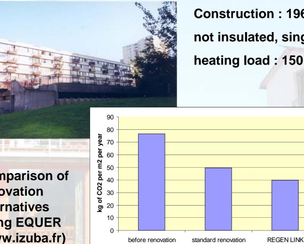
**Construction : 1969** not insulated, single glazing heating load : 150 kWh/m2/an
