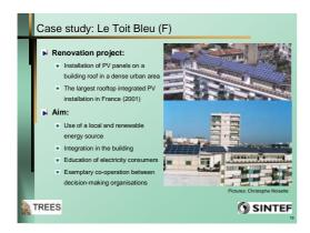
The roof area is completely covered by PV panels, amounting to a total area of 220m<sup>2</sup>. The panels are mounted on the roof of the building, oriented South, with an optimal inclination angle of 35°. In the project, polycrystalline PV cells were used, with a theoretic efficiency of 13%.
