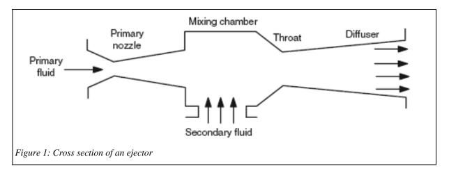
The primary fluid is accelerated in a converging-diverging nozzle, creating a pressure drop in the mixing chamber, which has the effect of drawing the secondary fluid. The two fluids are then mixed and a shock wave may take place in the following zone (throat in Figure 1). This results in an increase in pressure of the mixture and reduction of its velocity which becomes subsonic. The diffuser then converts the residual velocity into increased pressure.
