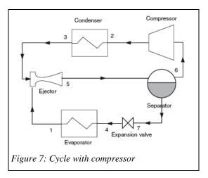
vapor and to slightly recompress it. The two-phase mixture is separated at the ejector outlet and the liquid enters the expander and then the evaporator. The vapor stream is compressed to 12 bar and then condensed in a slightly subcooled liquid state.
